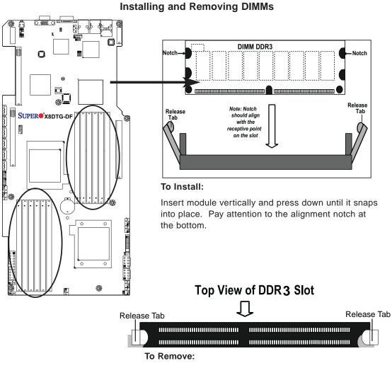
Use your thumbs to gently push the release tabs near both ends of the module. This should release it from the slot.
